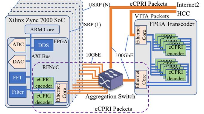
Fig. 5. The Schematic of Fronthaul Logical for eCPRI.
